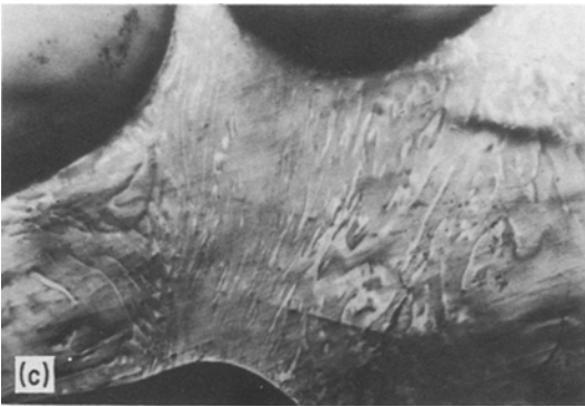
Figure 4 Microphotographs of coke surface obtained by the co-carbonization of heat-treated SRC pitch. (SRC410) with H-A240, HTT: 580°C; (a) SRC410 (as prepared), (b) SRC410, and (c) SRC410 with H-A240 (60 wt %).
