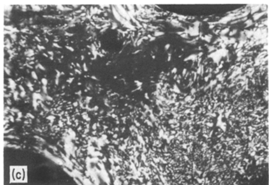
Figure 5 Microphotographs of coke surface obtained by the co-carbonization of SRCmeso420 with partners. Amount of partner: 60 wt%, HTT: 580°C; (a) SRCmeso420, (b) SRCmeso420 with A240, and (c) SRCmeso420 with H-A240.
